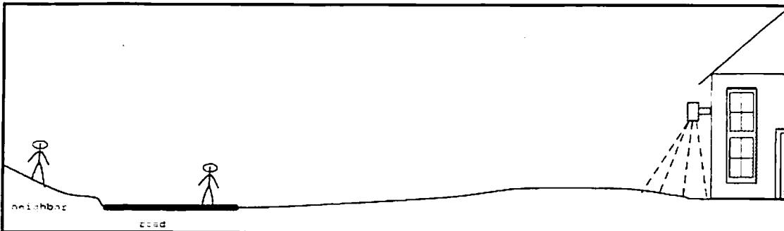
A low wattage (preferably yellow) bulb is shielded by a non-translucent hood/shade which only allows the light to project downward. The fixture is focused directly on the area to be lit, minimizing illumination of the wall of the house and the surrounding landscape. The bulb is not visible beyond the property line or from a roadway.
