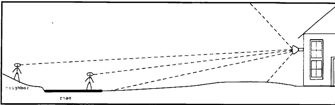
The glare of the bright flood light is visible to neighbors, motorists and people on the road, and illuminates the night sky. "Glare" means the hot spot of the bulb itself, not the area it is illuminating.
