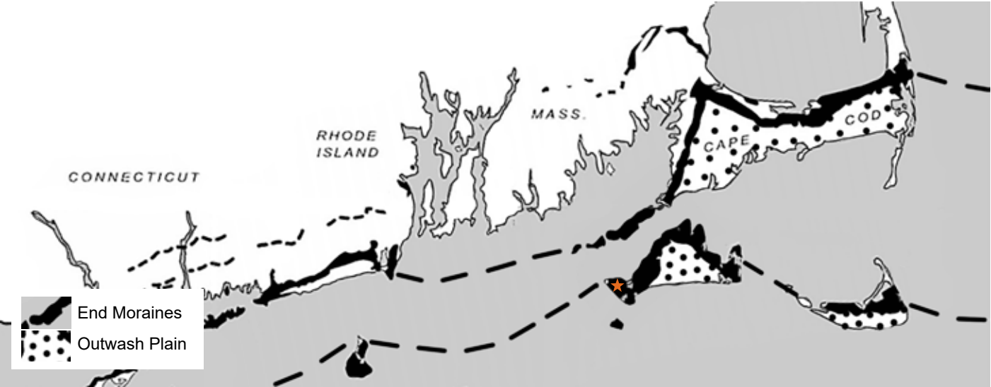
The end moraines of Martha's Vineyard and Nantucket mark the maximum southern extent of the Laurentide ice sheet, roughly 21,000 years ago. End moraines, comprising mixed debris accumulated during the glacier's advance, are pushed in front of the glacier and deposited in heaps at the maximum extent. South of the end moraines, sandy outwash plains formed as meltwater streams spread and deposited sediments suspended in the glacier (USGS, 2008).
